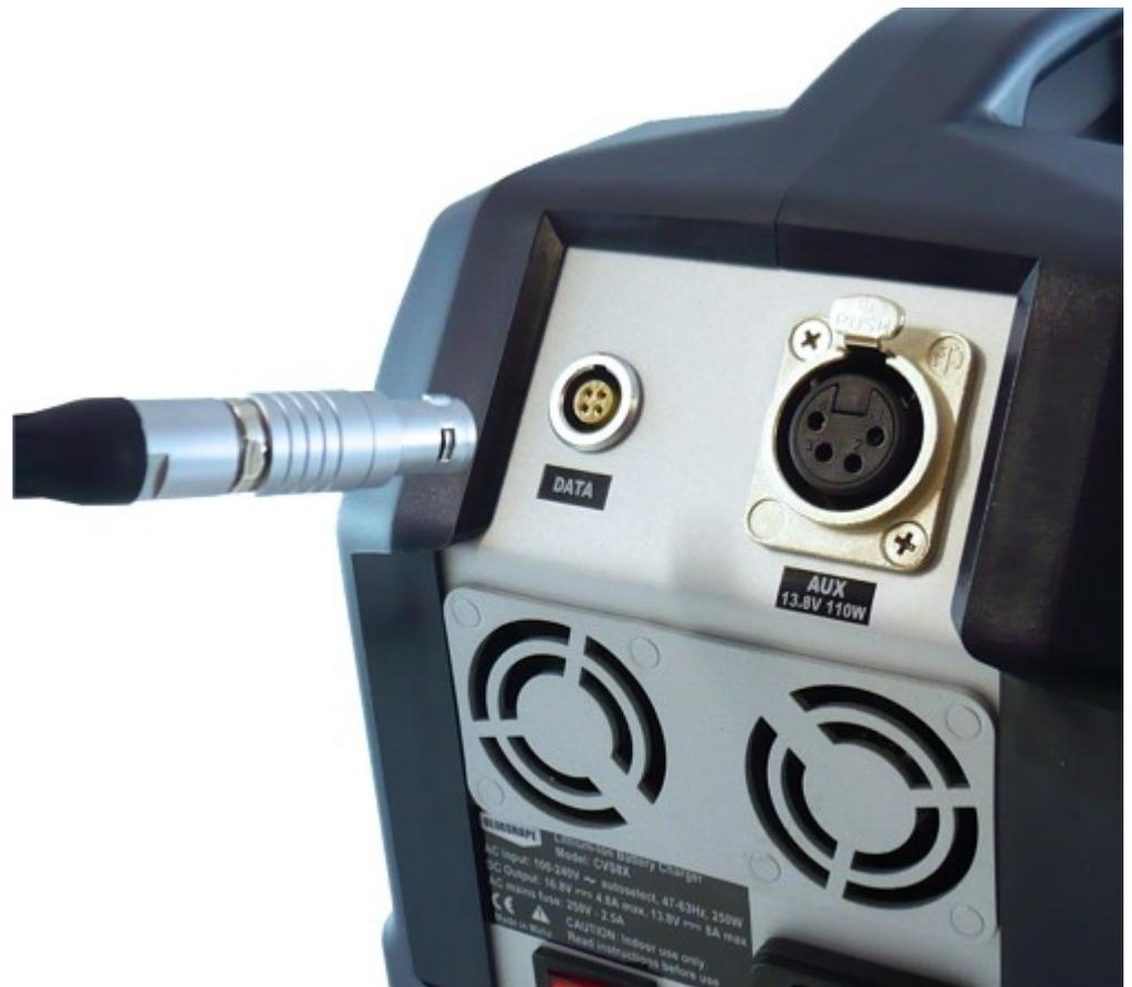
2. Plug the push-pull connector aligning the red dots
