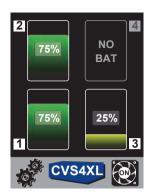
When no battery is connected or detected in a battery bay 'NO BAT' is shown in the battery status.
