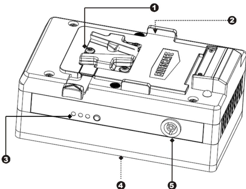
1. Installation interface for external V-Lock battery
