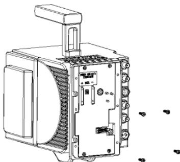
3. Figure shows lower Alu spacer part fixed to camera. Note the 2 large terminals (+ve) and (-ve) and the tiny data connector that now need to be connected to the wires on the main body of MVQUICKAL
