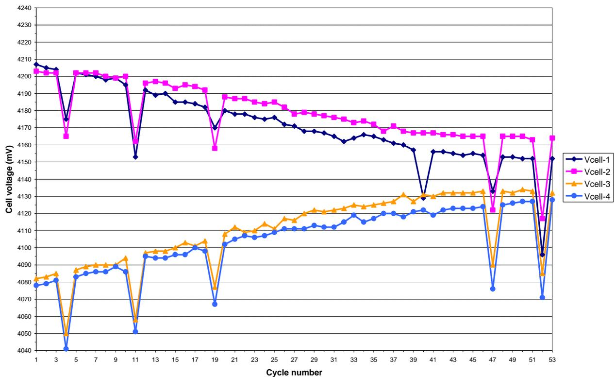
Cell#3 and cell #4 have a voltage much lower than the others do. If this situation is not corrected, any subsequent cycle could lead to a more severe unbalance, self-incrementing cycle after cycle, with a fast drop of pack performance and a premature termination of service life.
